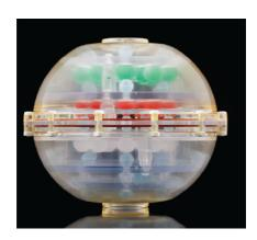
CaliberMRI provides MRI phantoms with calibration solutions and tissue mimics that have traceability up to and including full SI traceability through NIST when available.
