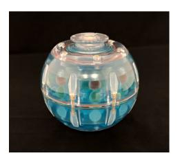
CaliberMRI provides MRI phantoms with calibration solutions and tissue mimics that have traceability up to and including full SI traceability through NIST when available.
